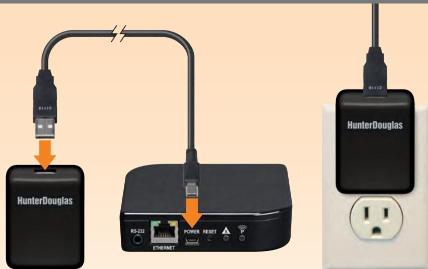
Connect the USB power supply cable to the power supply and Gateway.
