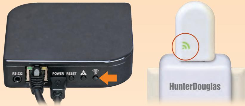
Press the **P** button on the back of the Platinum™ Gateway. The light on each Platinum Repeater should turn GREEN.
