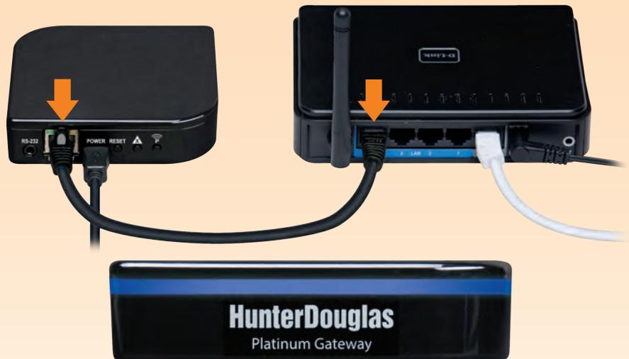
Connect the Ethernet cable to the Gateway and an open LAN port on your router. The light on the front of the Platinum Gateway will flash RED while it boots up and then change to a solid BLUE.
